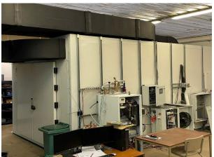
Measurement of thermal conductivity of building materials using the guarded hot plate method and parallel hotwire method (ISO83O2, NBN B62-2O1 and NBN B62-2O2)
