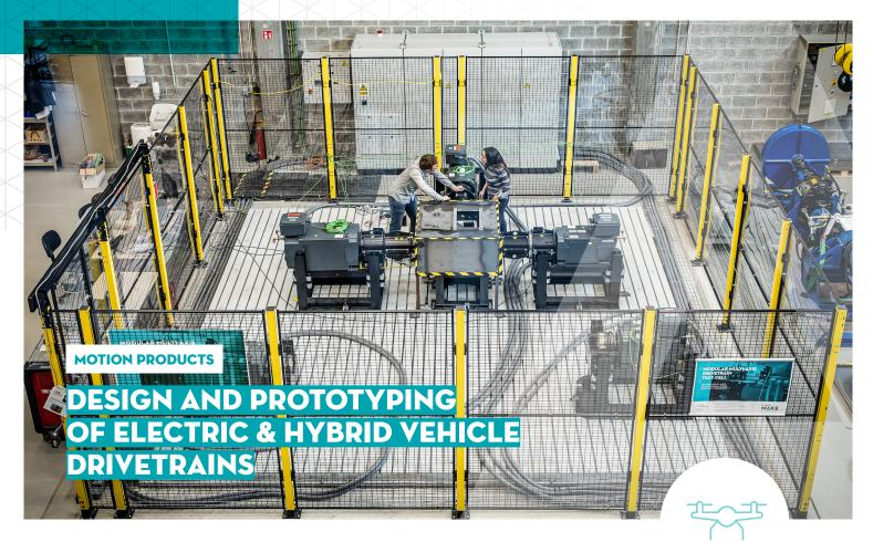
Flanders Make designs and prototypes electric and hybrid vehicle drivetrains in terms of energy consumption, lifetime, costs and comfort. Using our simulation platform, we optimise the design and control architecture of these drivetrains. Furthermore, we integrate proof-of-concepts for validation on test vehicles in lab and road environments.
